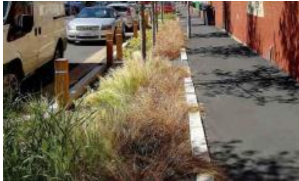
Figure 5-2: Typical Image of a Filter Strip
