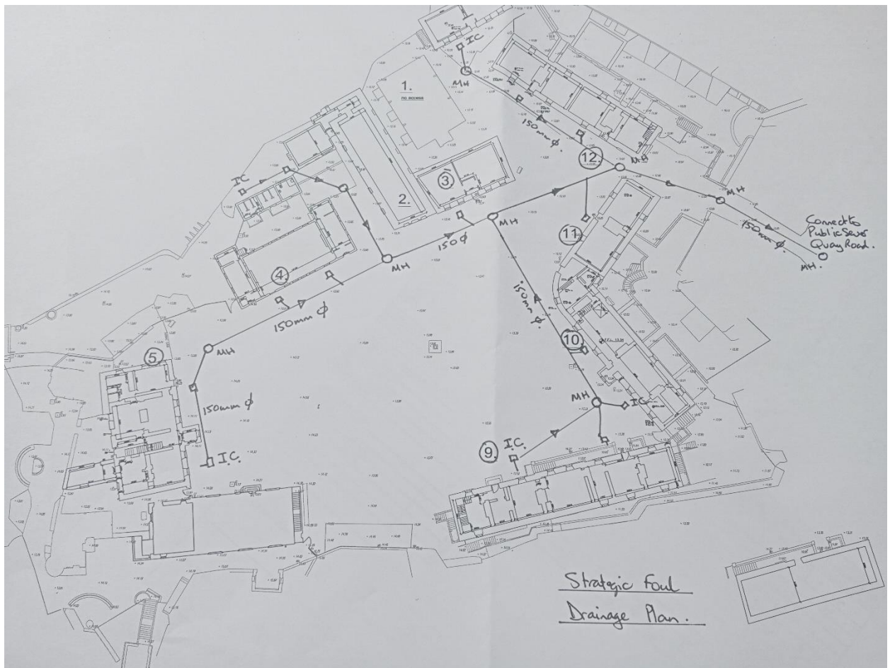
Figure 6-4: Indicative Proposed Foul Drainage Plan
