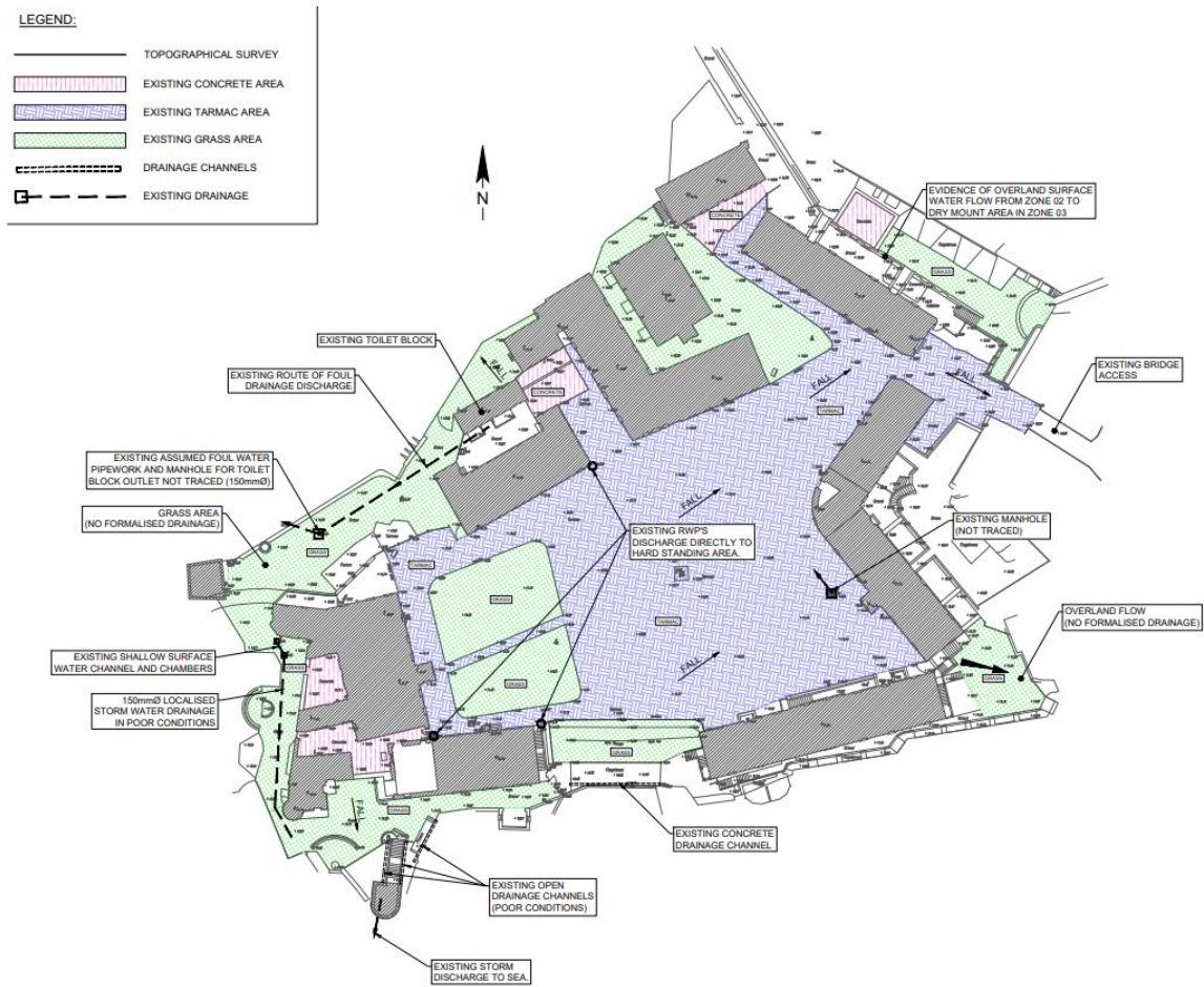
Figure 3-6: Existing Drainage Plan
