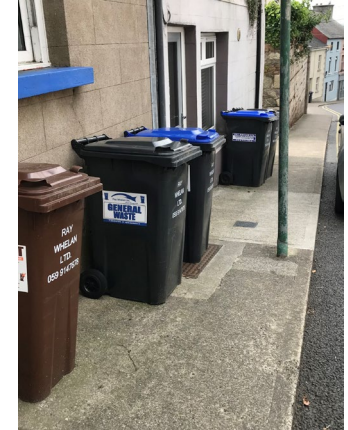
Narrow and discontinued footpaths, often without dished kerbs and hardly any tactile paving for universal access while bin refuge blocks access in many locations
