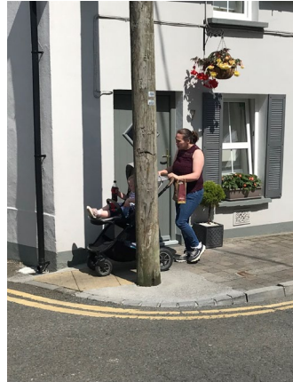
Narrow and discontinued footpaths, often without dished kerbs and hardly any tactile paving for universal access while bin refuge blocks access in many locations
