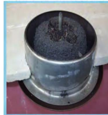
Fire Rated Ceiling Air Valve sealed after a fire
