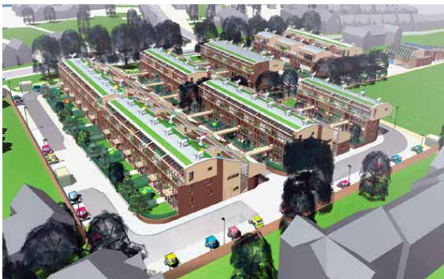
Left: 'BedZed' residential scheme, London. The site layout is planned to optimise orientation for solar gain.
