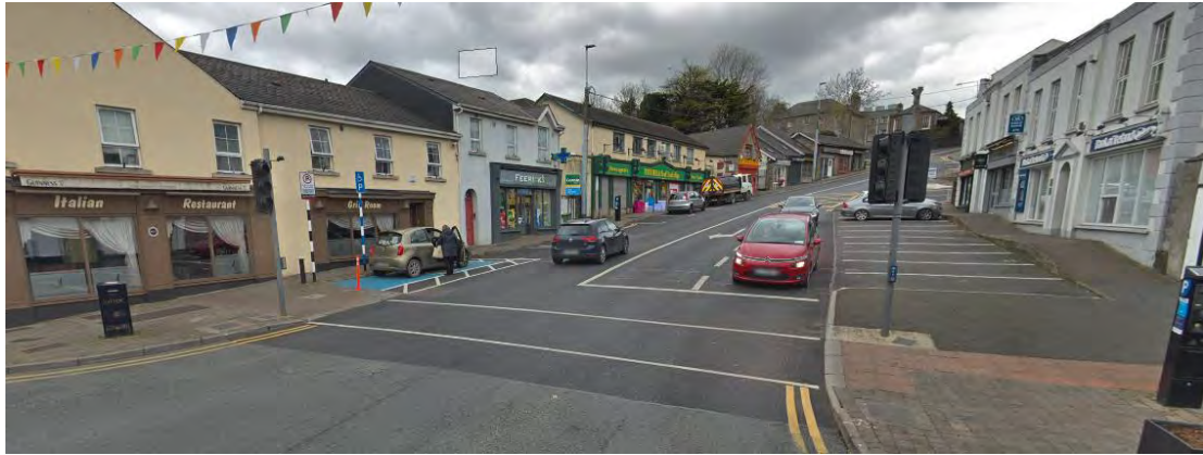
Plate 5.15 Main Street/ Captain Hill Three Way Signalised Junction, Leixlip. Note the proximity of the parallel parking spaces to the traffic signal. Vehicles must often reverse park into tight spaces at this location.
